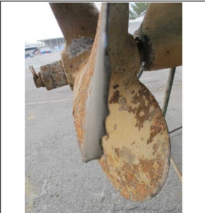
Props are damaged
